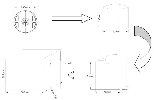
Note:5 meters/reel, 1reel/antistatic bag, 3 antistatic bags/box, 20 box/export carton;
